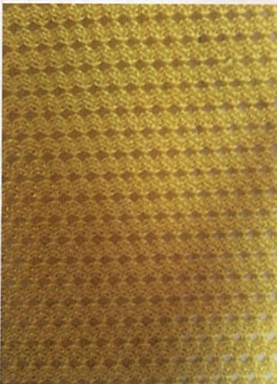
Cordura AFT (air flow technology) fabrics, developed by Tiong Liong
